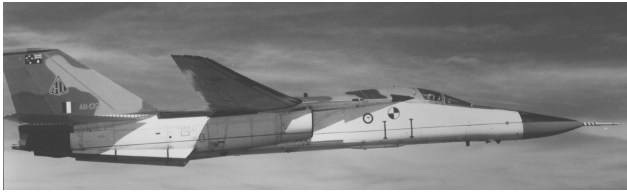
Fig. 1 General Dynamics F-111C variable geometry strike aircraft fitted with air data probe.
